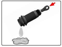
Drain the oil from the shock absorber.
