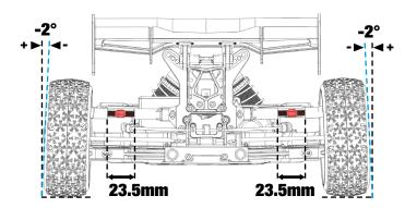
Adjust the angle by screwing the TURNBUCKLE.
