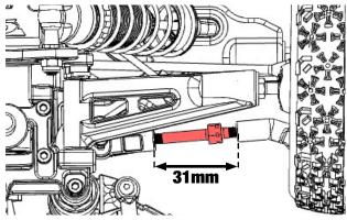
Adjust the angle by screwing the TURNBUCKLE.
